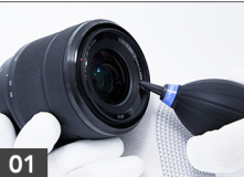
Use air blower to blow dust and away
