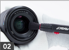
Use a cleaning pen to sweep away floating dust
